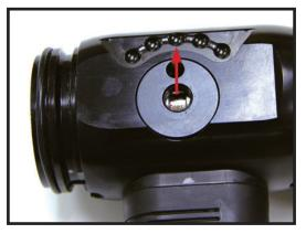
**Step 16)** Install the detent springs and balls back into the bail handle. Using the same method as when the handle was removed retain the springs and balls in the handle with your thumbs. Install the handle over the valve snapping it into place. Insure that the valve handle is oriented as indicated in the photo. The cam pin hole should be forward toward the exit of the nozzle.
