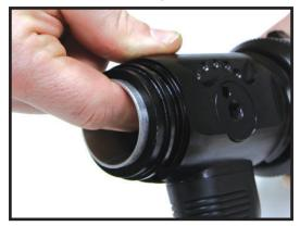
TASK FORCE TIPS LLC MADE IN USA • TFT.com 3701 Innovation Way, Valparaiso, IN 46383-9327 USA 800-348-2686 • 219- 462-6161 • Fax 219-464-7155 **Step 7)** Inspect the tapered leading edge of the slider. This is the edge that seals against the plug. If this edge is damaged replace the slider. (Part # G605)
