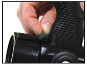
**Step 23)** With the valve in the closed position pour a cup of water into the valve. Check to insure no water leaks through. If it does the valve plug likely needs to be backed out a little further.
