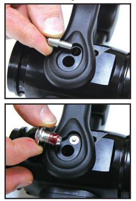
**Step 18)** With the valve handle held in the closed position, using the 3/16" Allen wrench back the valve plug out (unscrew) unit it makes firm contact with the slider. Once contact is made with the slider, open the valve handle part way and unscrew the valve plug 10 degrees. This will set the proper tension between the valve plug and slider.
