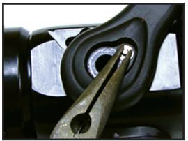
**Step 5)** Holding your thumbs over the detent balls and springs on the bail handle pull the handle upward and off using your thumbs to capture the balls and springs when the handle is removed.
