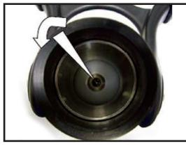
**Step 19)** Included with the kit is a new o-ring (VO-134) to seal the coupling to valve body connection. Lightly grease this o-ring. Install this o-ring on the valve body as shown Also, lightly grease the ball ring groove on the valve body.
